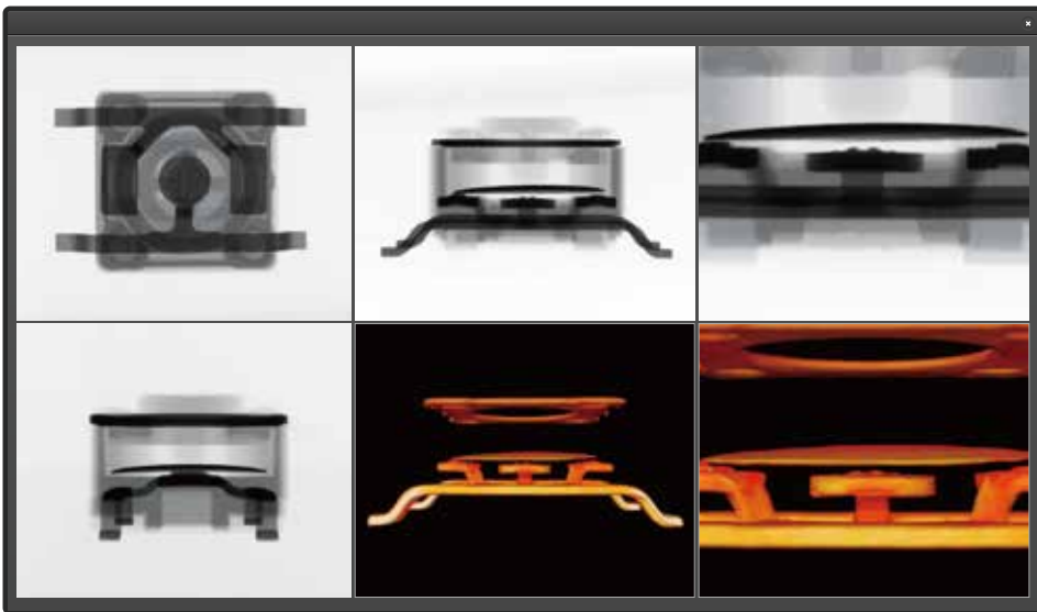
Switch 9 \mu\text{m} pixel size in ultra-high resolution mode.
